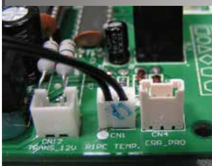
Compressor current protection
